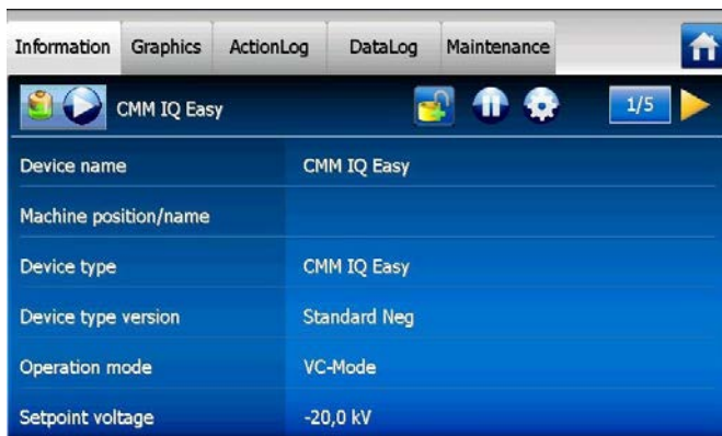
Figure 9, Changing CMM IQ Easy parameters
